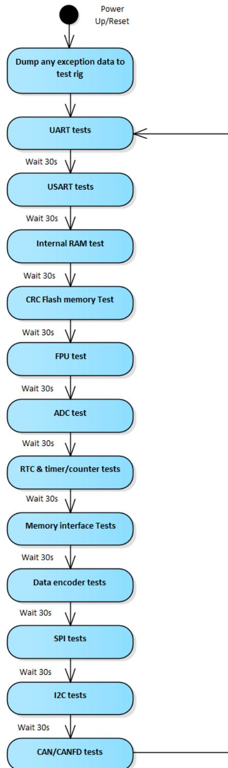
Figure 4: SAMV71 in test software loop
