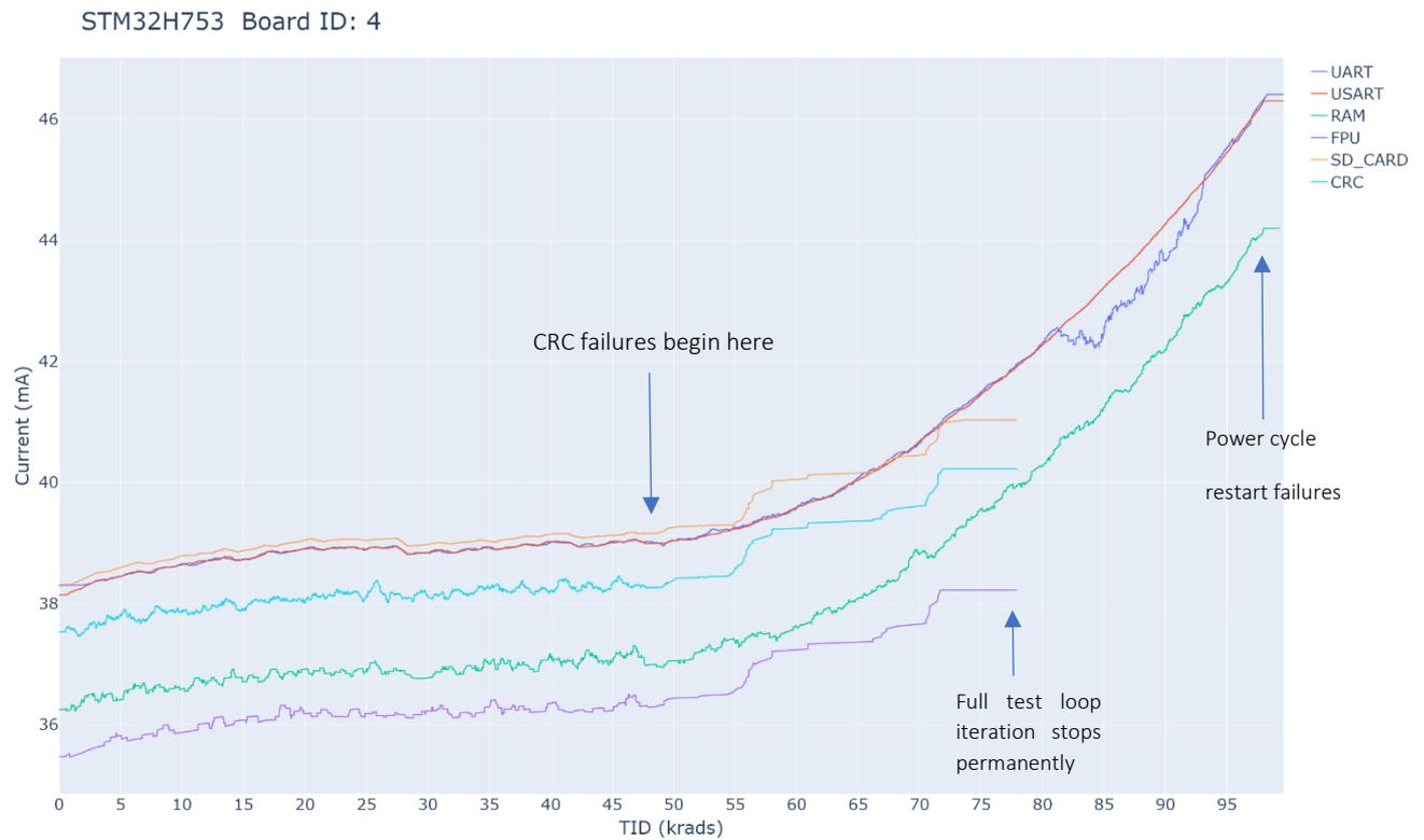
Figure 15: STM32 destruction test, current consumption for the all the tests conducted. The current begins to increase for all tests more rapidly when the CRC/flash memory failures begin to occur. The exceptions on the Flash integrity CRC test occur permanently at 78 kRads, meaning no further tests of the FPU or SD-CARD were conducted either.
