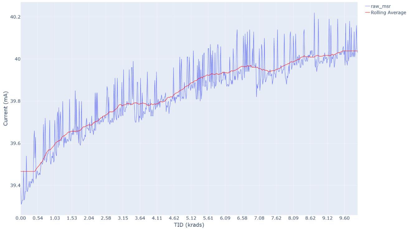
Figure 12: STM32 current consumption for the USART test on Board 3. This board was irradiated until mission specified test value of 10 kRads.
