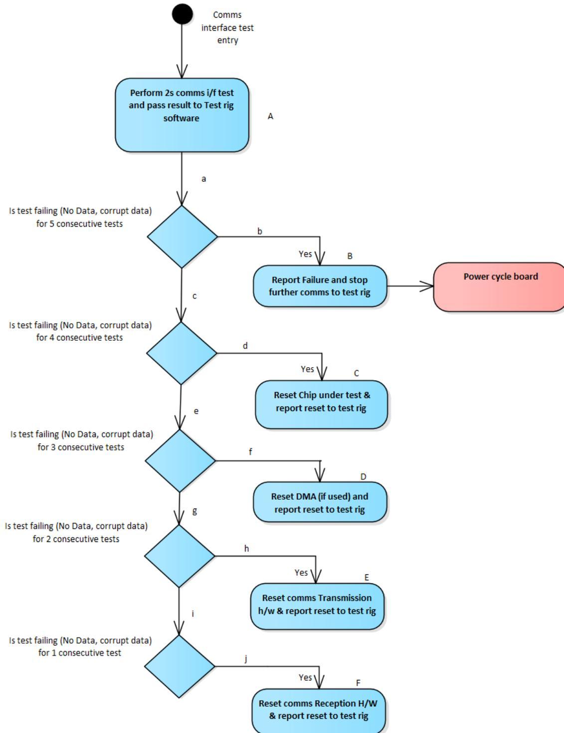
Figure 7: Automatic recovery from I/O interface errors
