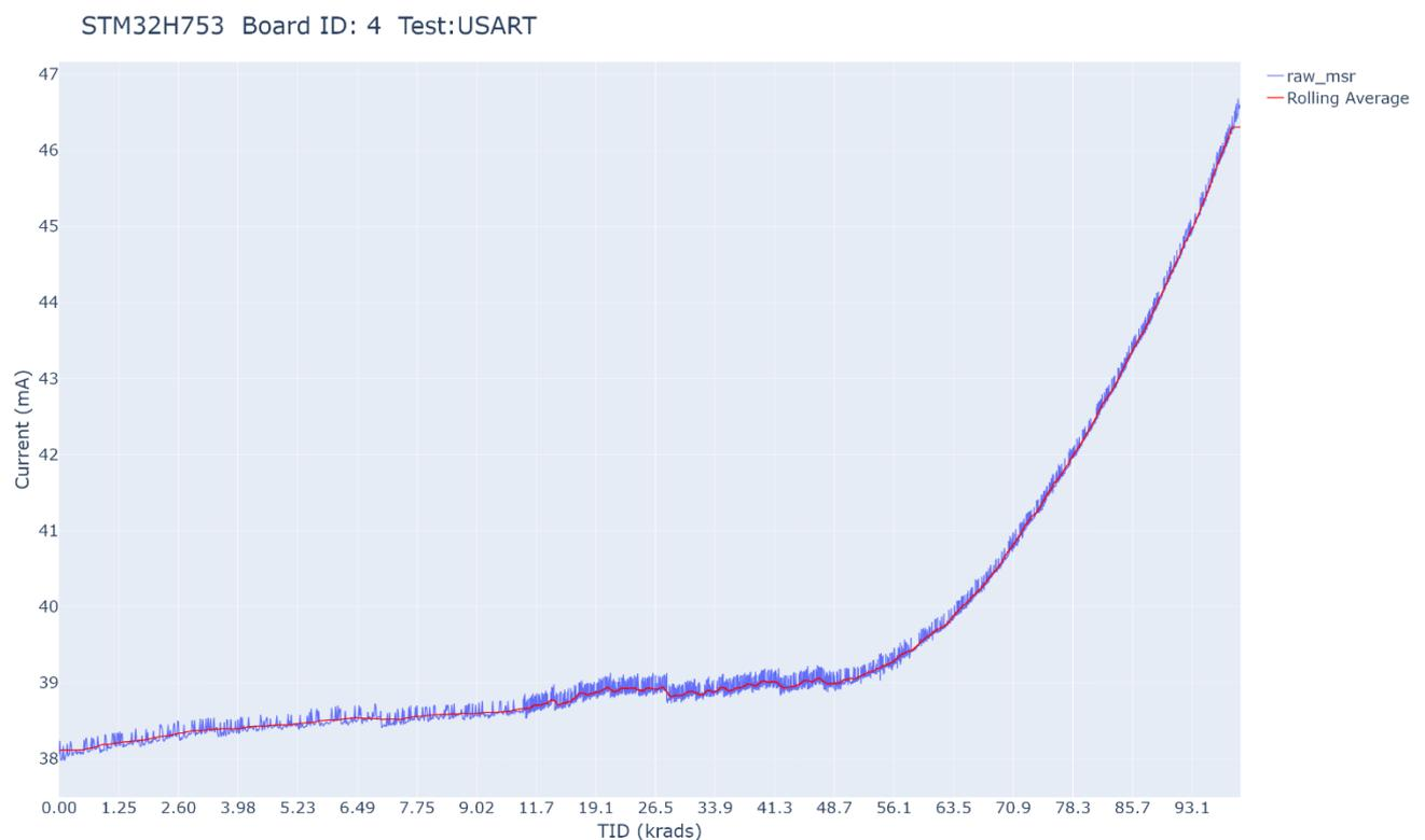
Figure 14: STM32 destruction test, current consumption for the USART test
