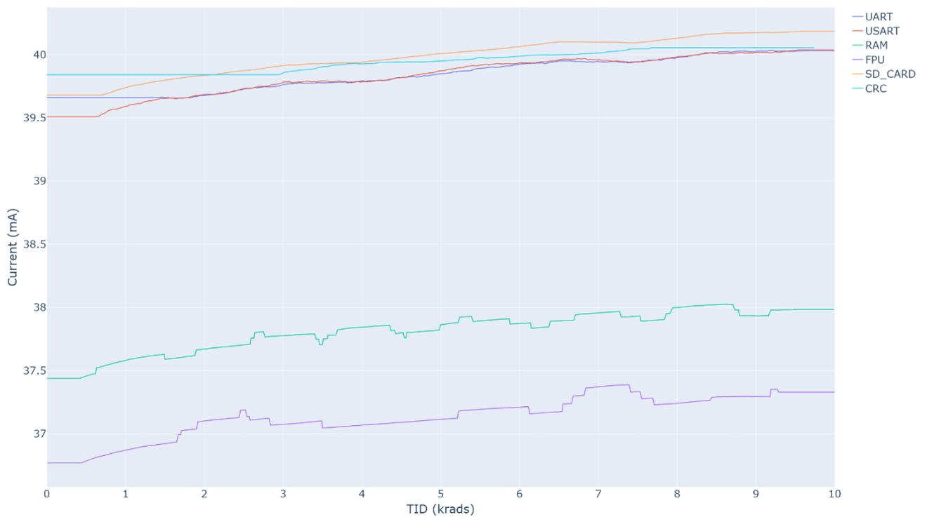
Figure 13: Current consumption of all tests conducted on STM32H753 board 3, up to a TID of 10 krad.
