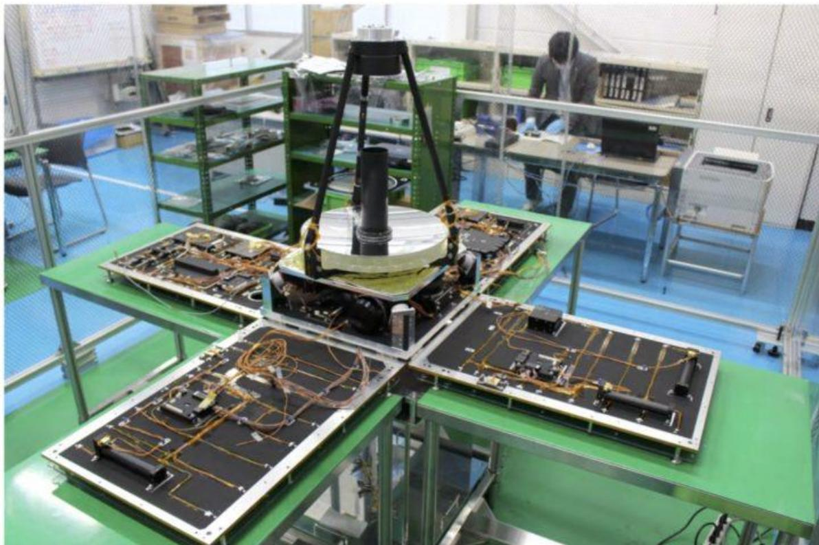
Figure 6-2: CE-SAT 1 partially assembled.
